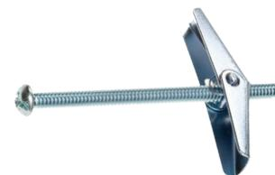
Toggle bolts are a hollow wall anchor designed for use in block, wallboard, plaster, plywood as well as other hollow base materials. Toggle bolts are a two-part assembly consisting of a machine screw and a wing toggle.
