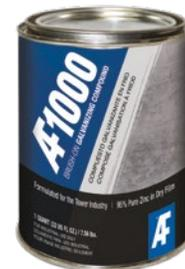
**AF1000** is a single package zinc rich coating. This coating contains 95% metallic zinc in the dry film to provide cathodic corrosion protection for iron and steel. Cold Galvanizing Compound is also excellent for the repair of worn or damaged galvanized steel. This product is not intended for use on rusted steel. **AF1000** meets the performance requirements of ASTM A-780-01 (par. 4.1.2, 4.1.3, 4.2.2).
