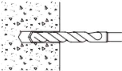
1. Using the proper diameter bit, drill a hole into the base material to a depth of at least 1/4" deeper than the required embedment. The tolerances of the drill bit used should meet the requirements of ANSI Standard B212.15. Blow the hole clean of dust and other material.
