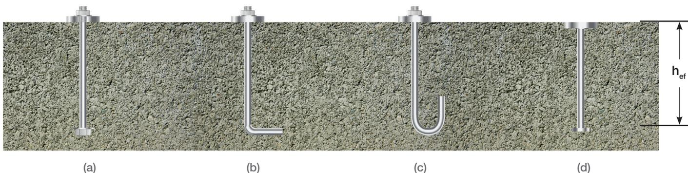
Cast-in anchors: (a) hex head bolt with washer; (b) L-bolt; (c) J-bolt; (d) welded headed stud.
