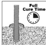
**9** Do not disturb, torque or apply any load to the installed anchor until the specified full cure time has passed. The amount of time needed to reach full cure is base material temperature dependent - refer to Table 14 for appropriate full cure time. Use caution not to exceed the maximum specified torque once the anchor has fully cured.
