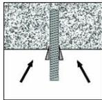
**8B** For overhead installations, horizontal and inclined (between horizontal and overhead), wedges should be used to support the anchor while the adhesive is curing. Take appropriate steps to protect the exposed threads of the anchor element from uncured adhesive until after the full cure time has elapsed.
