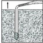
**7B** Piston plugs must be used with the extension tube attached to the supplied nozzle for horizontal and overhead installations with anchor sizes 5/8" to 1 1/4" diameter and rebar sizes of #5 to #10. Select the proper injection plug for the drill hole diameter as given in Table 13.
