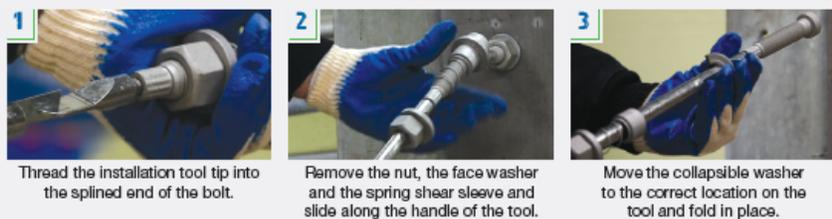
1 Thread the installation tool tip into the splined end of the bolt.
