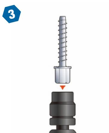
3. Select a powered impact wrench of a torque wrench, attach an appropriate sized hex socket to the wrench and mount the screw anchor head into the socket.
