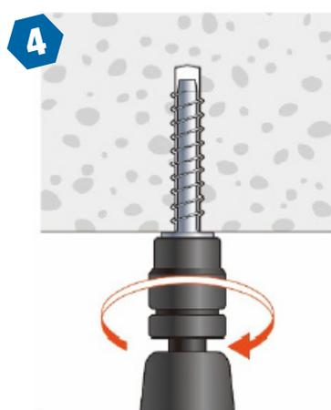
4. Install the anchor with an impact wrench through the surface. The correct force should be considered during the installation to make sure the socket doesn't do damage to the member surface or self-inflict any damage to its connecting threads.
