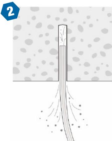
2. Remove dust and debris from the hole using a hand pump or compressed air.
