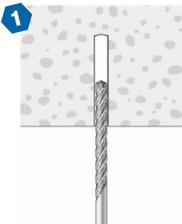
1. Drill a hole into the base material to the required depth using a drill bit that meets the requirements of ANSI B212.15.
