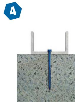
4. Using drill, hammer mode disabled, drive the anchor through fixture and into hole until nut driver spins free from head of anchor.
