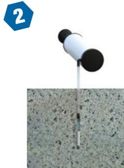
2. Clean hole with compressed air or vacuum to remove any excess dust/debris.
