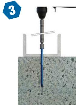
3. Place XCS setting tool with drive socket over drill bit.
